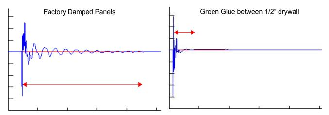
What you see is the vibration resulting from each panel being struck with an impact hammer. The faster the vibration decays, the better the damping. In both cases, the frequency in question is ~100Hz, or very close to the resonance in the walls shown above. The damping of the Green Glue sandwich is no less than 5 times higher, and this despite the fact that the factory damped panels tested have 2 damping layers, not just one.
